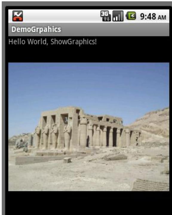
This control can be linked to an image file. The image file must be in /res/drawable-x, the directory /res/drawable-hdpi will work with lower resolution devices. The file ramasseum.png has been copied across in the example above.
